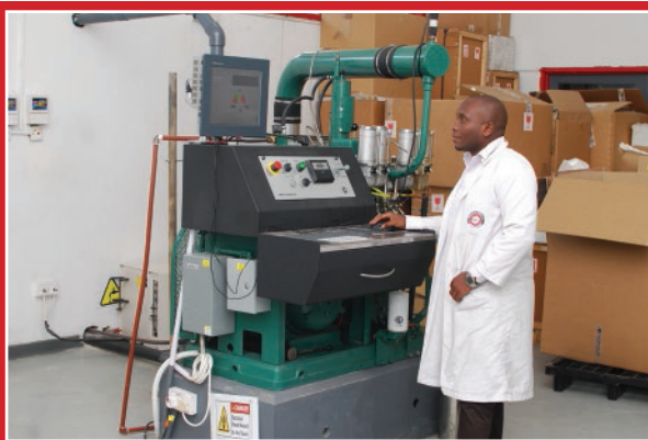
Testing of Research Octane Number (RON) in petrol in the Chemistry Laboratory.
